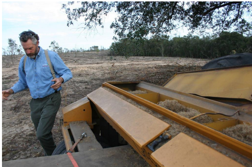
The Grasslander planter distributes seed mix over the bare ground for forest restoration. Pulled by a tractor, the Grasslander measures the amount of seed that is spread and its tires push the seed into the sandy soil to help them germinate. Longleaf pine seedlings are planted by hand during the process. Photo by Bruce Ritchie.
